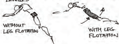
SKETCH #8 - SWIMMER WITH FLOTATION ADDED TO THE LEGS, CHANGING THE SIGNATURE SO LESS ENERGY NEEDED TO BE LEVELLED
